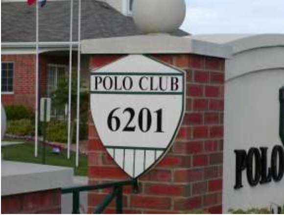
Address of Complex: Minimum 5 inch high, ½ inch stroke
